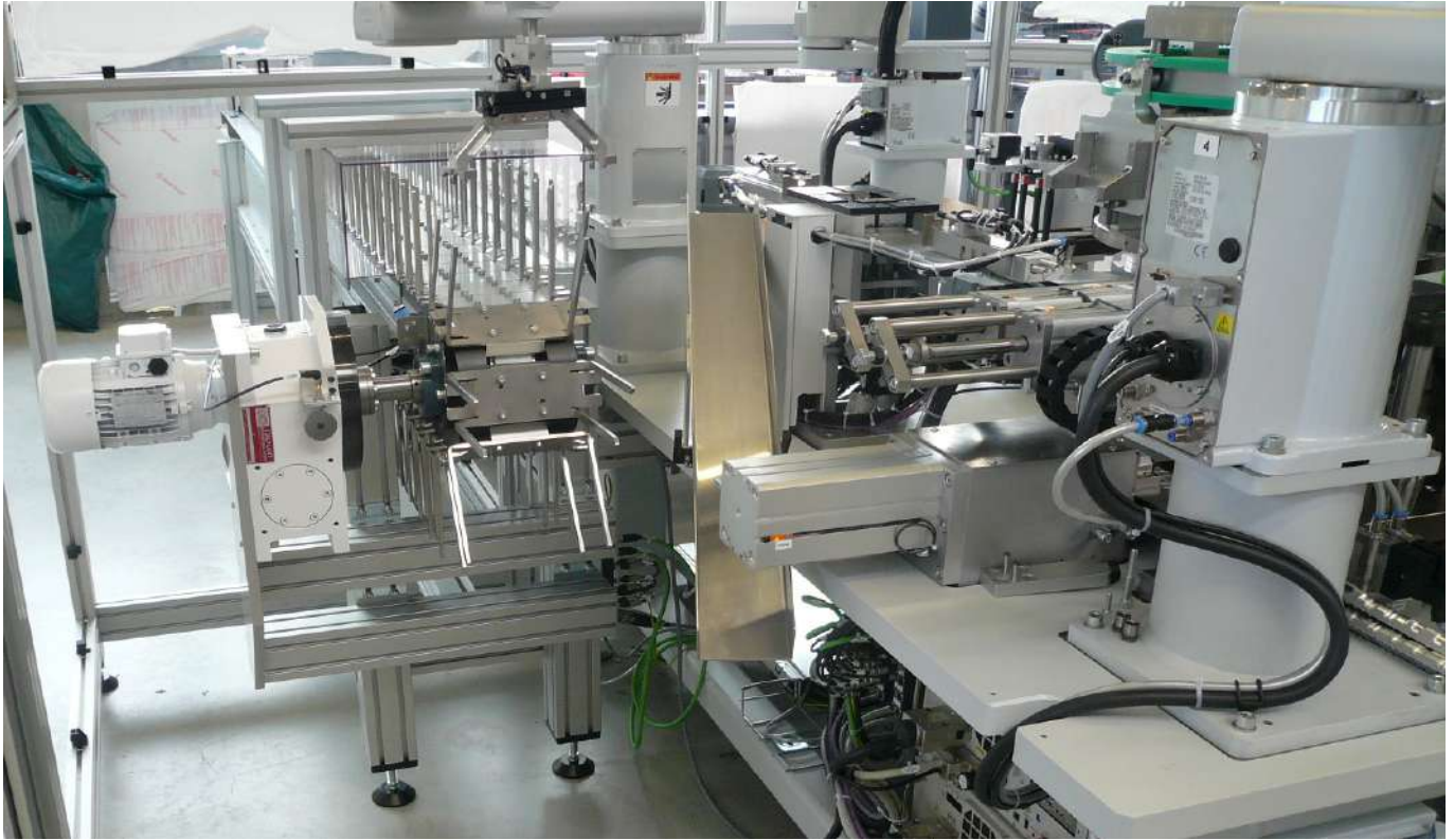
PBC 80 x 1000 mm - Drawer guides assembly
